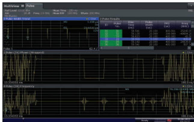
▲ Fig. 6 The unique pulse signal can be isolated and analyzed completely using the R&S FSW-K6 pulse measurements option.
