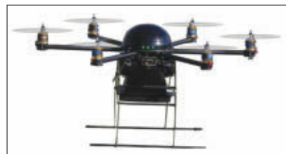
▲ Fig. 11 TiaLinX UAV with UWB radar sensor (courtesy of TiaLinX).
