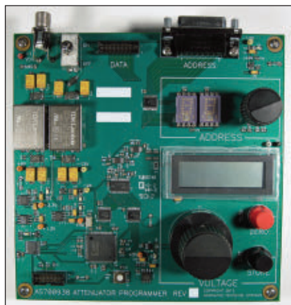
▲ Fig. 1 Programming board for programming attenuator driver.
